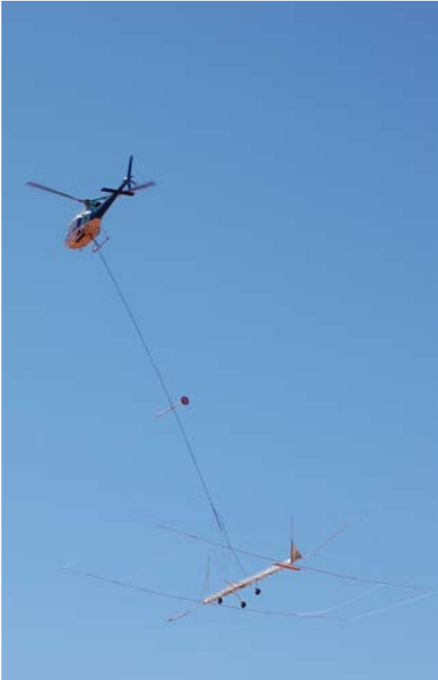
Figure 2 Electromagnetic loop slung below helicopter during surveying.
