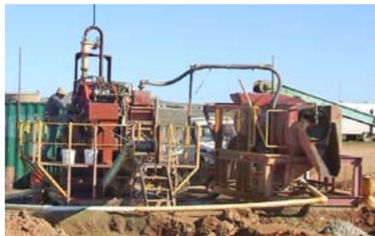
Figure 2 Bulk sampling treatment plant.
